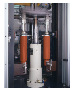
Shock absorber rig in operation at Federal-Mogul Technology center during test of GLYCO® 298
